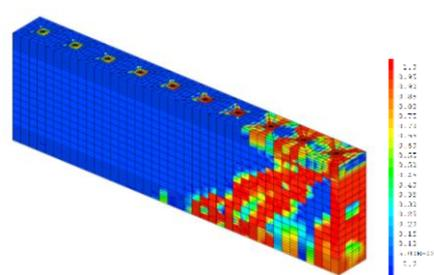
**Figure 22:** Damage distributions of the concrete in the SP1-1 beam, case (4)
