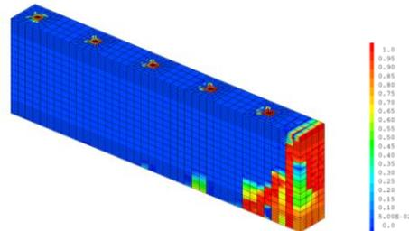
**Figure 26:** Damage distributions of the concrete in the SP1-2 beam, case (6)
