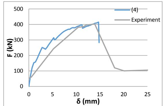
**Figure 18:** Comparison of the shear force - displacement curves of SP1-1 beam for case (4) and experiment
