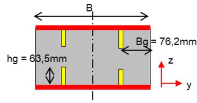
Figure 7: Schema of the transversal section of SP1 beams
