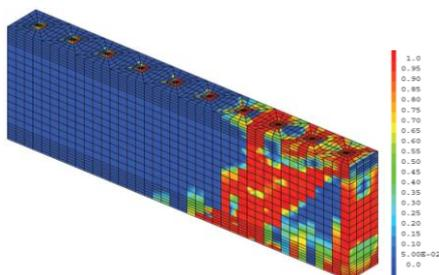
**Figure 21:** Damage distributions of the concrete in the SP1-1 beam, case (3)
