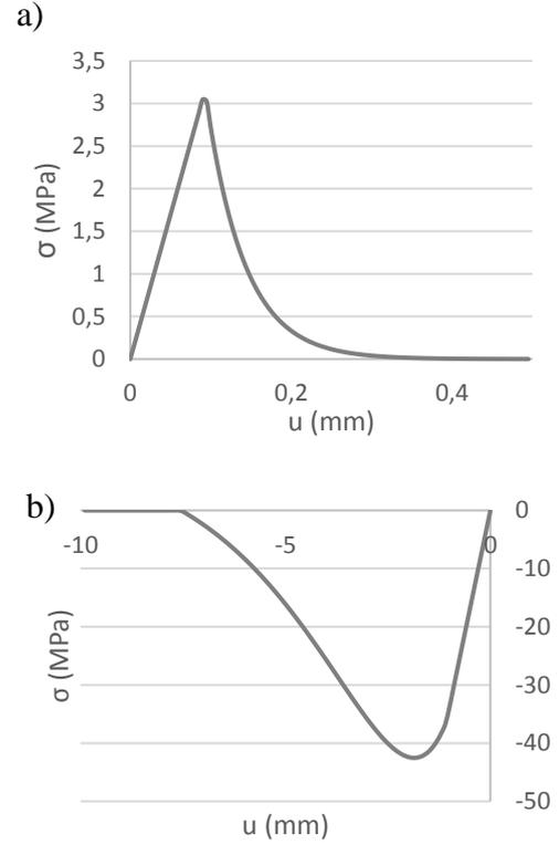
**Figure 10:** Simulated concrete behavior a) in tension, b) in compression
