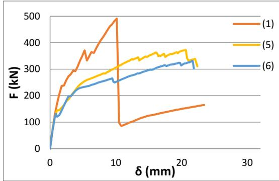
**Figure 23:** Shear force - displacement curves of the SP1-1 beams for the case (1), (5) and (6)
