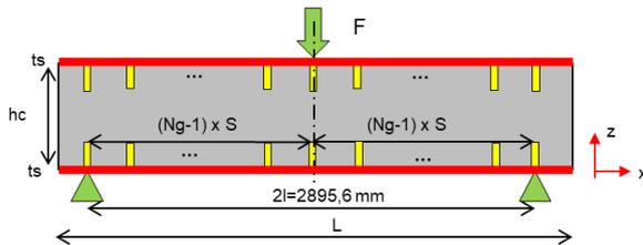
Figure 6: Schema of SP1 beams
