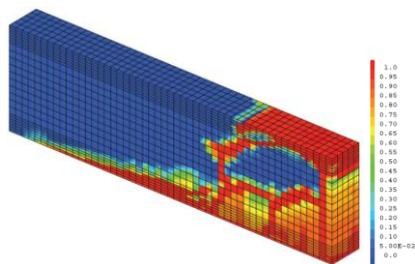
**Figure 19:** Damage distributions of the concrete in the SP1-1 beam, case (1)
