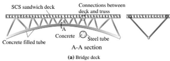
**Figure 2:** Schema of a SCS sandwich deck [14]
