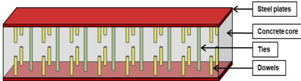
**Figure 1:** Schema of a SCS structure with dowels and ties
