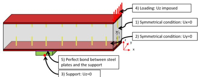
Figure 14: Boundary conditions on the beams
