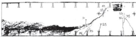
Figure 12: Crack pattern of the concrete of the SP1-1 beam [2]
