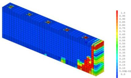
**Figure 25:** Damage distributions of the concrete in the SP1-2 beam, case (5)
