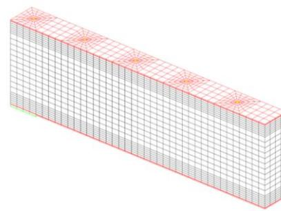
Figure 9: Mesh of SP1-2 beam
