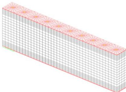
Figure 8: Mesh of SP1-1 beam
