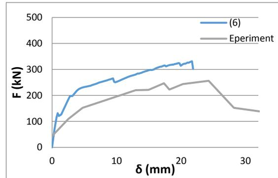
**Figure 24:** Comparison of the shear force - displacement curves of SP1-2 beams for case (6) and experimental results
