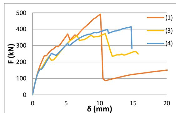
Figure 17: Shear force - displacement curves for cases (1), (3) and (4)
