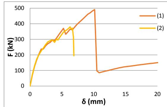
Figure 16: Shear force - displacement curves of the SP1-1 beams for the case (1) and (2)
