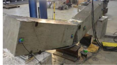
Figure 13: Failure of the SP1-2 beam [2]
