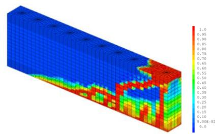
**Figure 20:** Damage distributions of the concrete in the SP1-1 beam, case (2)
