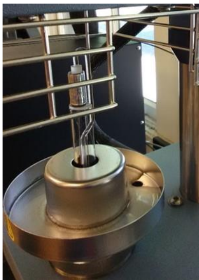
Figure 3: Photo of the cement paste sample inside the furnace of the TMA
