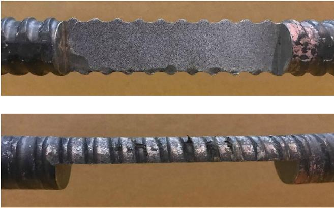
**Figure 1:** Cutting half of the cross section of the rebar by laser cutting
