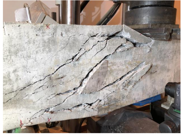
Figure 8: Crushing and spalling of surface concrete
