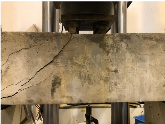
Figure 7: Shear failure of reference beams
