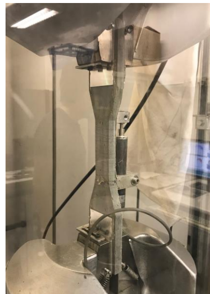
Figure 1: Direct tension test set-up for SHCC
