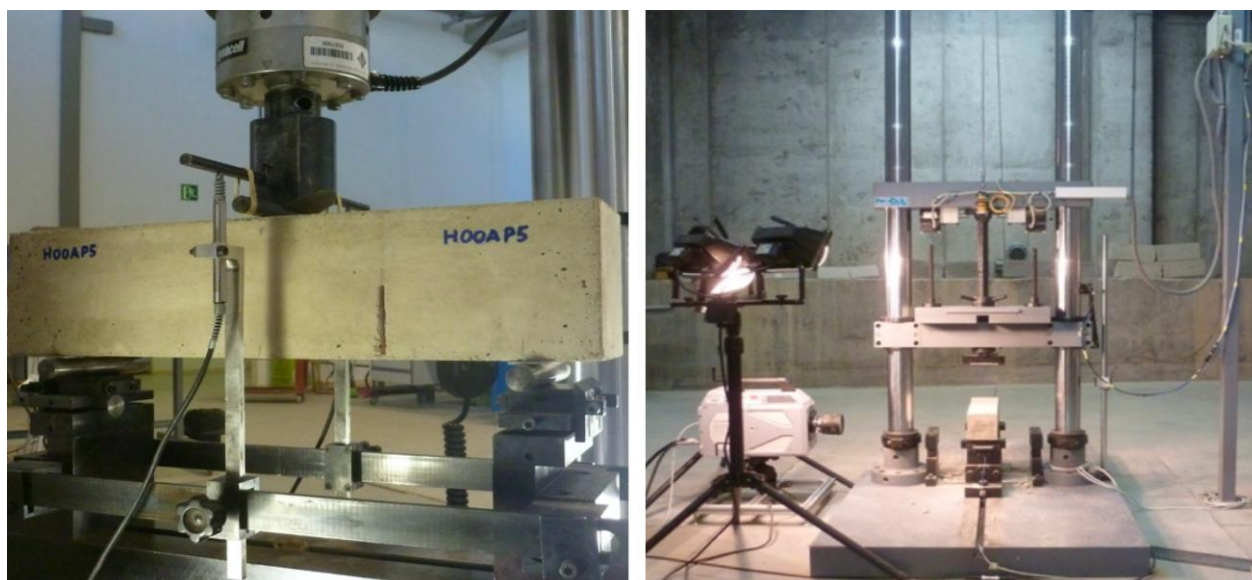
Figure 1. Specimens ready to be tested in the servo-hydraulic machine (left) and the drop-weight test device (right).
