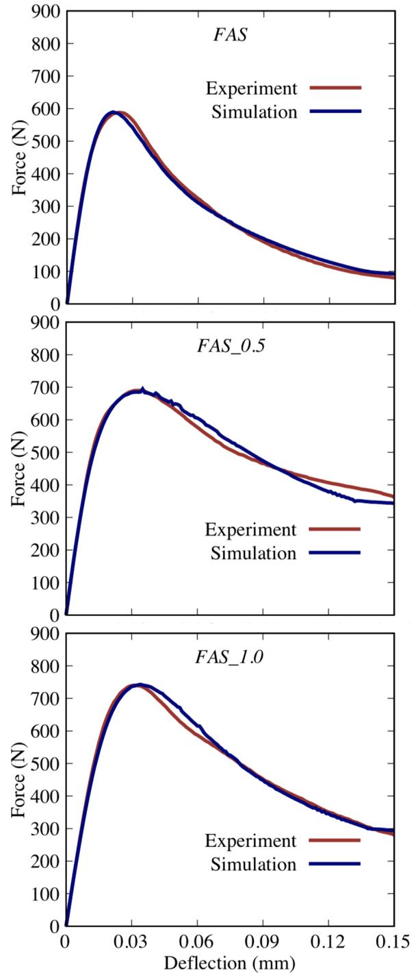
**Figure 10:** Selected  $F-d$  diagrams of FAS composite: experiment vs. numerical simulation.
