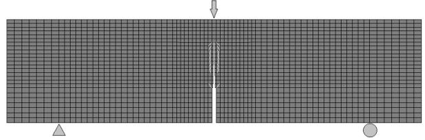
**Figure 3:** FEM model of the three-point bending test adopted for numerical simulations, including damage distribution at peak load.
