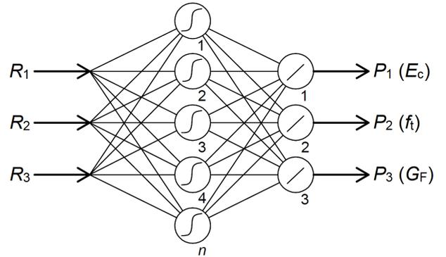
**Figure 7:** Diagram of the utilized feed-forward multilayer network.
