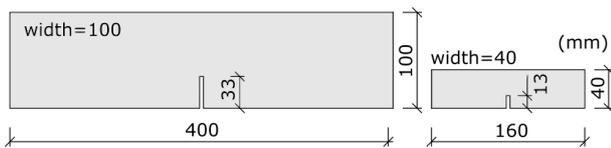
**Figure 1:** Typical specimen size for coarse-grained composites (left) and fine-grained composites (right) used in a three point bending fracture test.
