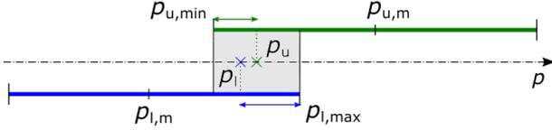
**Figure 8:** The calculation of weight factors for specimens in the overlapping area of two subspaces.
