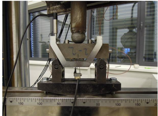
**Figure 2:** Fracture test configuration.
