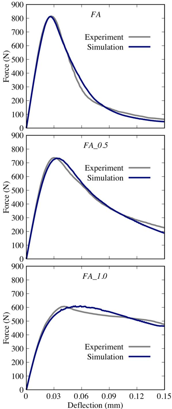
**Figure 9:** Selected  $F-d$  diagrams of FA composite: experiment vs. numerical simulation.
