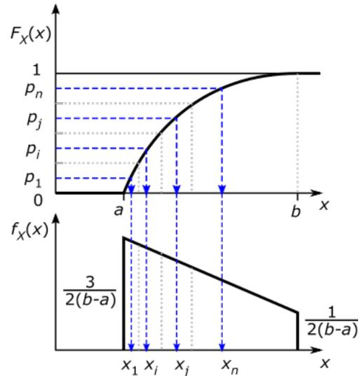
**Figure 4:** Generating random samples of the specific fracture energy, which has descending trapezoidal probability distribution.
