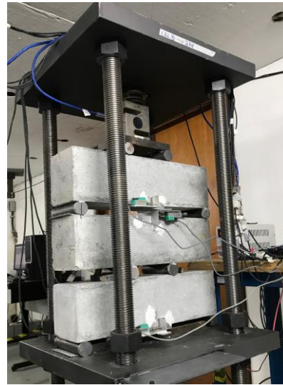
Figure 2: Flexural creep test setup.
