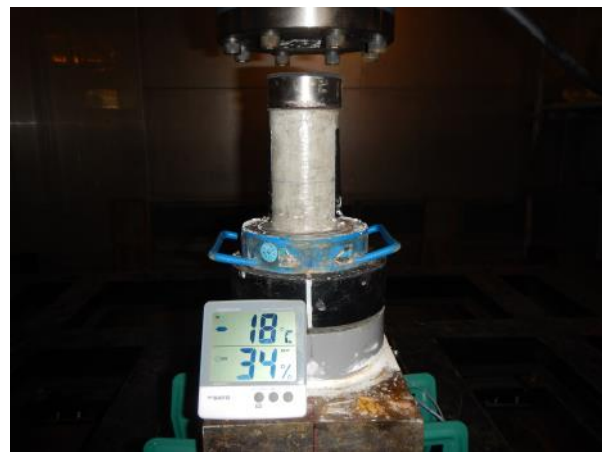
Figure 2 Loading test at low temperature
