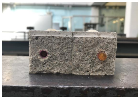
Figure 4: Polyurethane hardened inside Model 1 capsules embedded in the cement mortar matrix.
