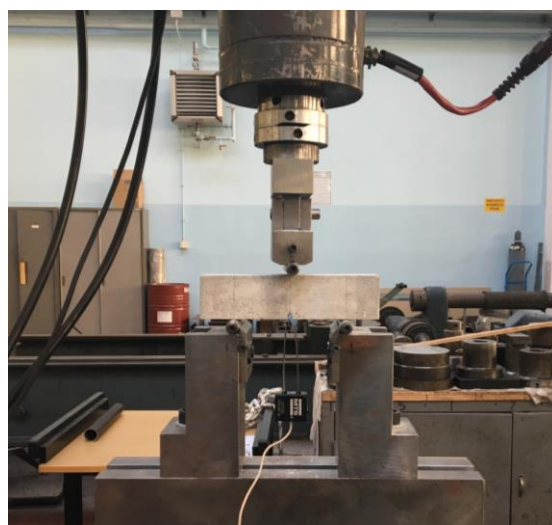
Figure 7: Specimen during the pre-cracking phase.
