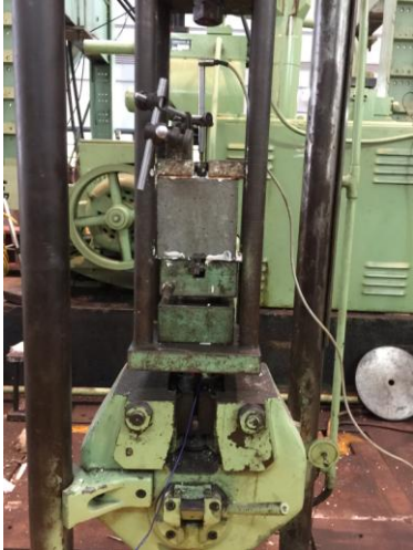
Figure 2: Test set-up for Pull out Loading
