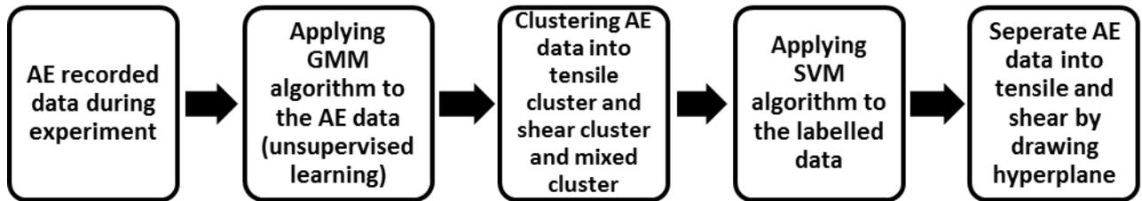
**Figure 1:** Schematic representation of crack classification procedure
