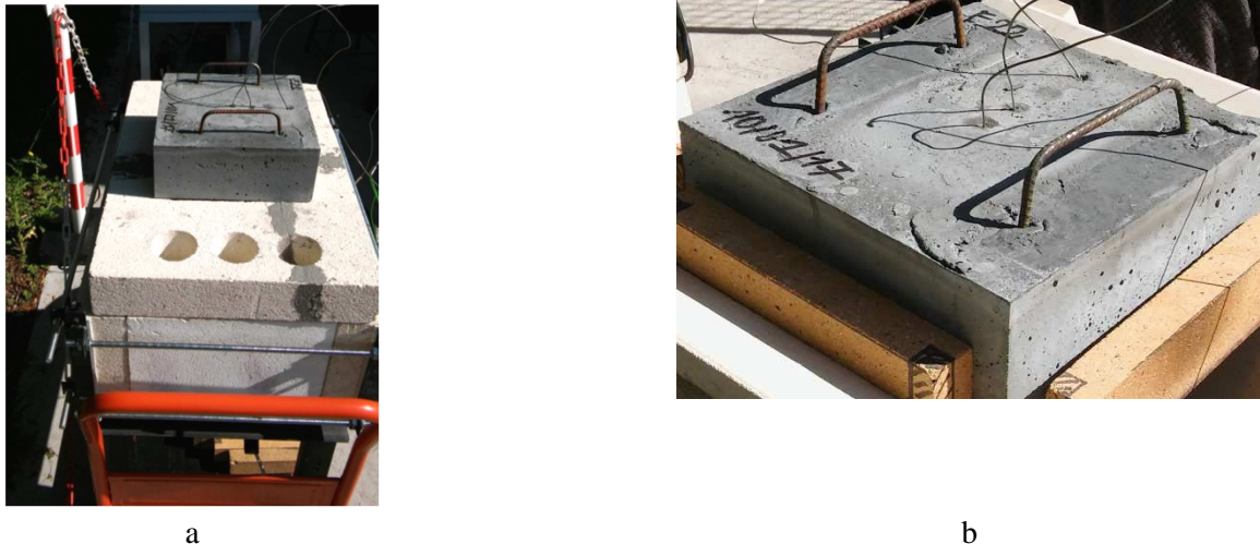
Fig.2. Photo of a- a global view of the spalling test bench and b- a detailed view of the specimen equipped with the three thermocouples.
