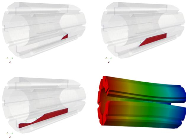
Figure 2: Progression of keyway root crack driven by internal stresses.
