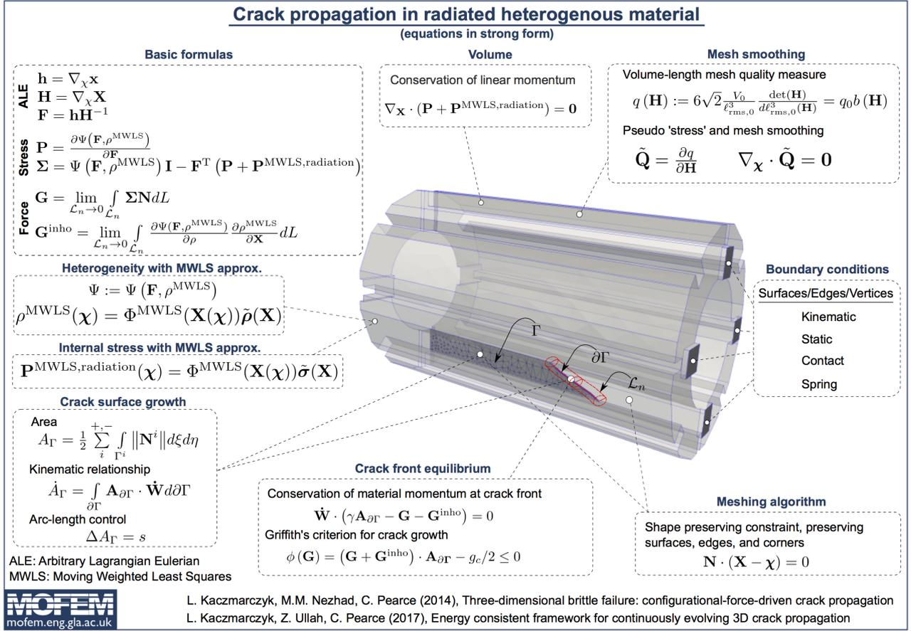
Figure 1: Equations for crack propagation in the radiated graphite, i.e. brittle heterogeneous material with internal stresses.
