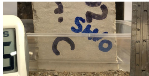
Figure 4. Concrete specimen with a natural crack face in a bath of cyanoacrylate
