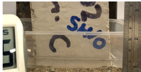
Figure 4. Concrete specimen with a natural crack face in a bath of cyanoacrylate
