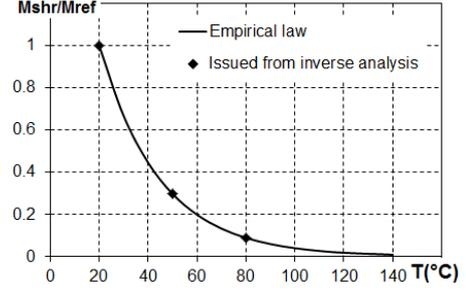
Figure 7: Evolution of  $M_{shr}$  according to temperature
