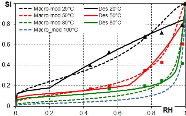
Figure 6: Desorption isotherms at  $\neq T$  °C
