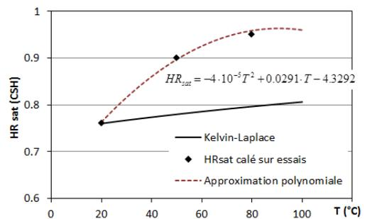
Figure 5: Effect of T on  $RH_{CSH,sat}$
