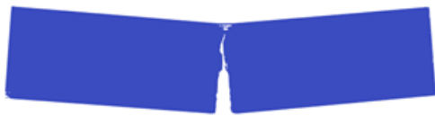
Figure 11 Failure mode for three point bending test
