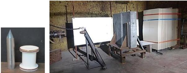
Figure 6. Projectile and experiment configuration
