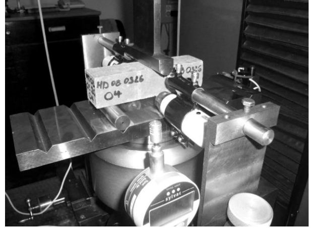
Figure 3: Experimental setup of the three-point bending experiments from VUT Brno [6].
