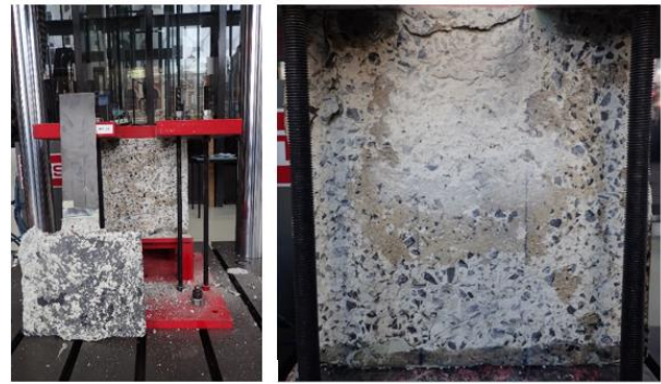
Figure 19: Mode of failure of the anchored model observed in the experimental work.
