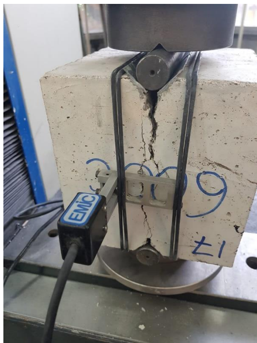
Figure 4: The roller-specimen interaction after DEWS test.
