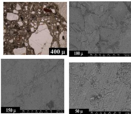
**Figure 5: Recycled concrete CPN G water quenched. Cracks widening and detachments along the RCA and NA interface (top-left). Multiple cracks within Si-bearing aggregates in the air cooled CPN G (top-right). Long cracks (bottom-left) and crack branching in the water cooled CPN G (bottom-right).**
