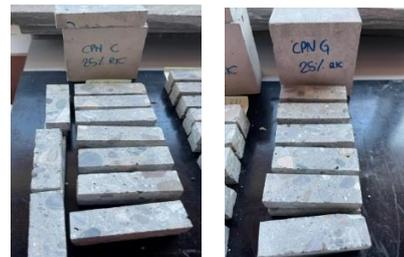
Figure 1: Recycled concrete specimens CPN C (left) and CPN G (right).
