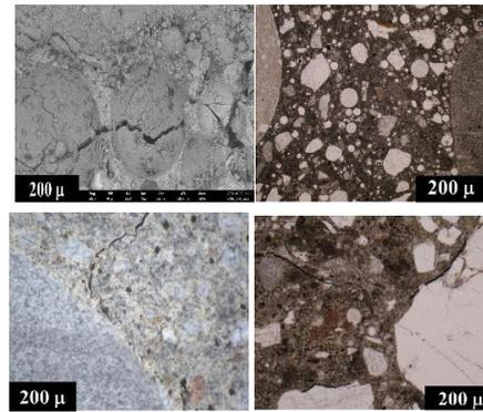
**Figure 4: Recycled CPN C exposed to 500 oC and water quenched. Aggregates and interface cracking (top-left). CPN G reference specimens with a dense microstructure (top-right) and macrocracking in the air cooled CPN G (bottom-left). Widening of the cracks and microcracking in the water quenched CPN G specimens (bottom-right).**
