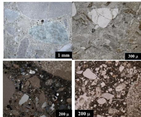
**Figure 2: Recycled concrete specimens CPN C top-left and top-right), CPN C air cooled (bottom-left), CPN C water quenched (bottom-right).**
