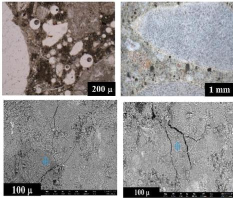
**Figure 3: Recycled CPN C exposed to 500 oC and water quenched (top-left). Grain pull outs of the water quenched specimens (top-right). Cracking of a Si-bearing aggregate and location of the SEM-EDX analysis (bottom-left).**
