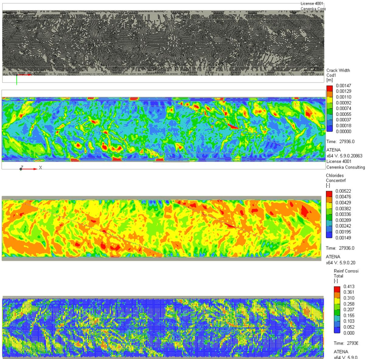
**Figure 9:** Numerical results at the bottom surface of the bridge deck after a 75-year-long chloride attack: (from top) Crack pattern, crack width, chloride concentration at the level of bottom reinforcement, and reinforcement corrosion degree. The crack pattern displays only cracks exceeding 0.25 mm.
