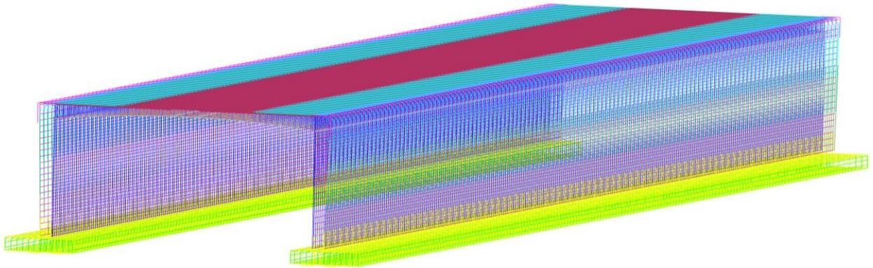
Figure 5: Layout of the discrete reinforcement bars in the model.
