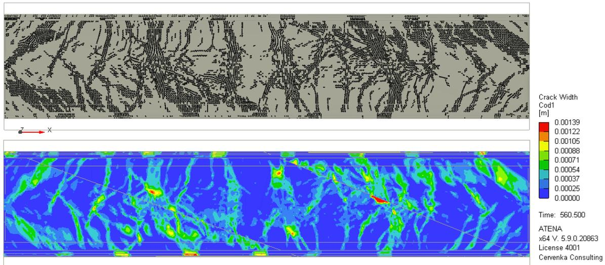
**Figure 8:** Numerical results at the bottom surface of the bridge deck after finishing the construction process: (top) Crack pattern, and (bottom) crack width. The crack pattern displays only cracks wider than 0.25 mm.
