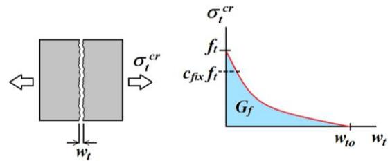
Figure 1: Crack opening law controlling the softening in the tensile branch of the material model.
