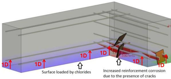
**Figure 7:** Schematic illustration of how mechanical crack accelerates the chloride penetration and thus the corrosion process.
