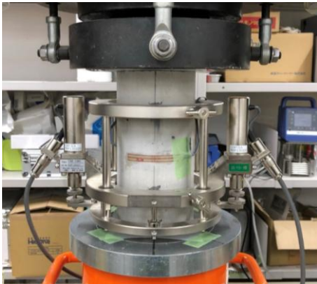
(a) Photo of compression test
