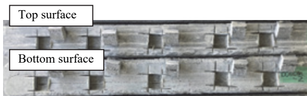
Figure 13: Fractured specimens for bond strength tests.
