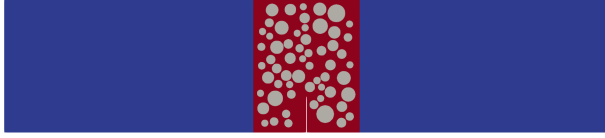
Figure 3: Mesostructure generated in three-point bending specimen
