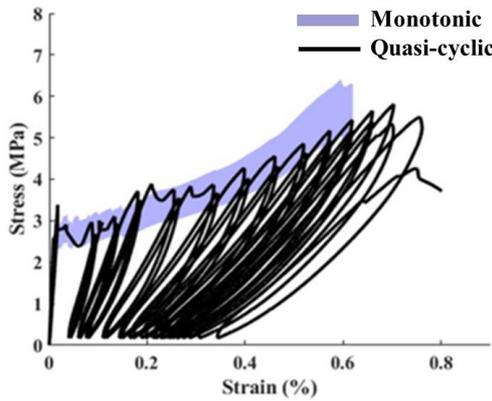
Figure 4. Typical stress-strain response under quasi-cyclic loading
