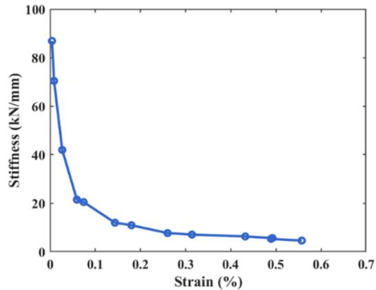
Figure 5. Stiffness degradation as a function of strain
