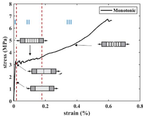
Figure 1. Typical stress-strain response of TRC under monotonic loading
