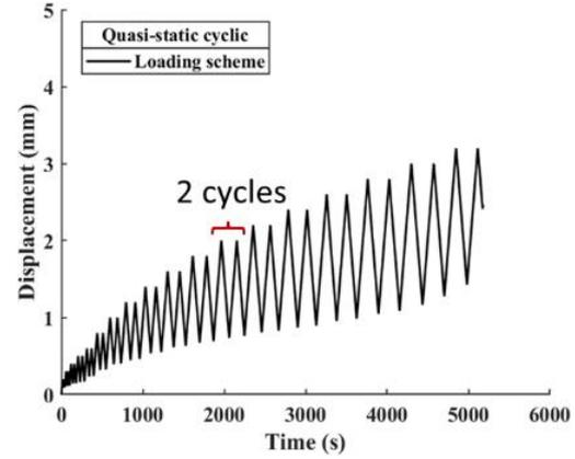
Figure 3. Schematic loading scheme
