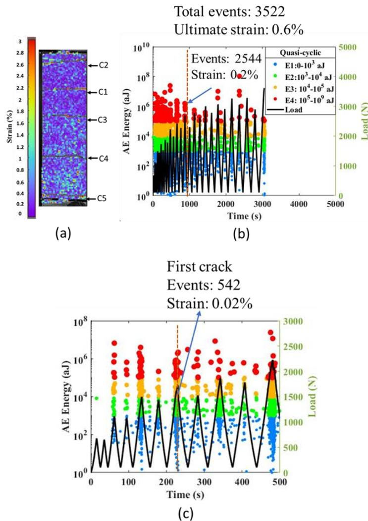
**Figure 6.** Energy evolution and crack formation of TRC under quasi-cyclic loading obtained from AE and DIC techniques
