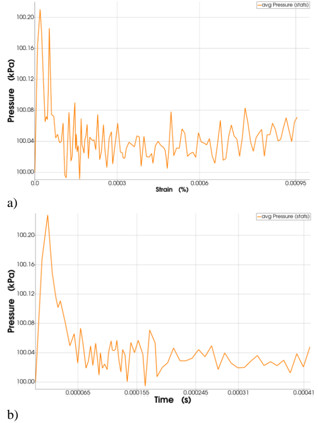
Figure 6: Coupled DEM-CFD results for fully fluid-saturated concrete specimen ( \alpha_q=1.0 ) with unbreakable aggregate: evolution of average pore fluid pressure [Pa] against vertical normal strain \varepsilon_y during dynamic uniaxial compression (a) \dot{\varepsilon}=50 1/s and b) \dot{\varepsilon}=100 1/s [5].
