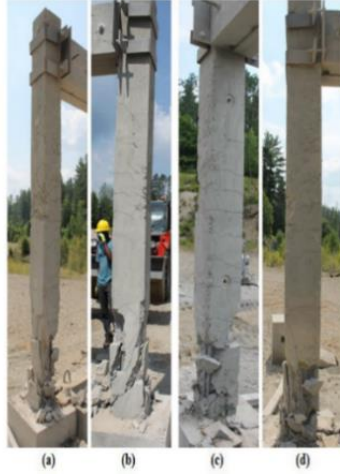
Figure 2: Experimental Post-Blast Damage [19]
