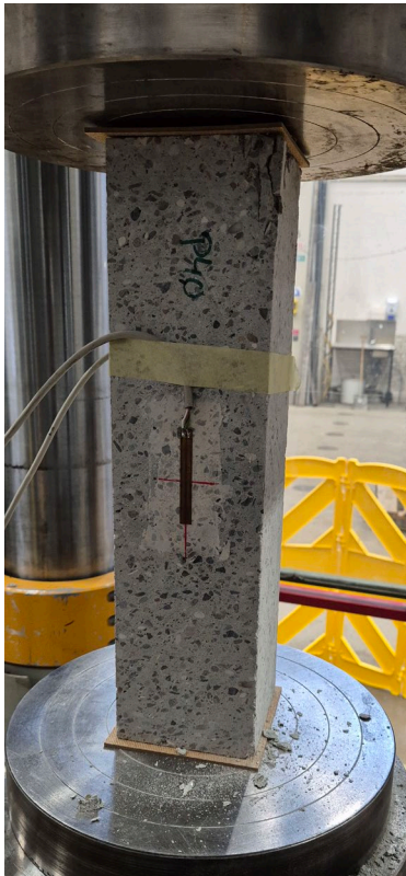
Figure 3: Specimen equipped with strain gauges, installed in test machine.
