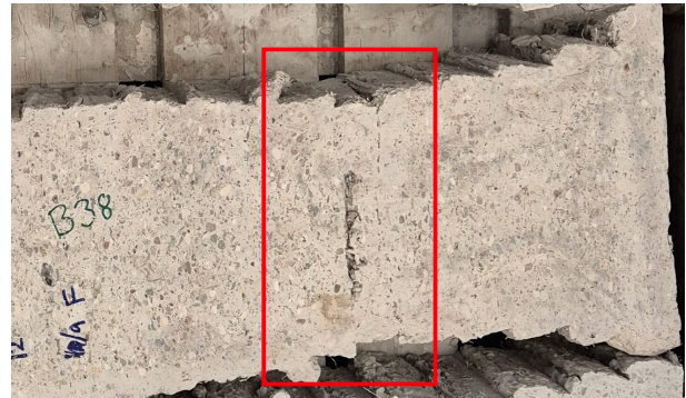
Figure 6: Example of significant flaw originating from issues in the print process.
