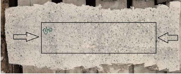
Figure 2: Printed material with indication of a typical specimen size, cut out from the 3D printed block.
