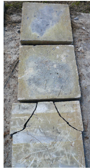
Figure 6: Slabs after one of the tests. From bottom to top, concretes A, B and C.
