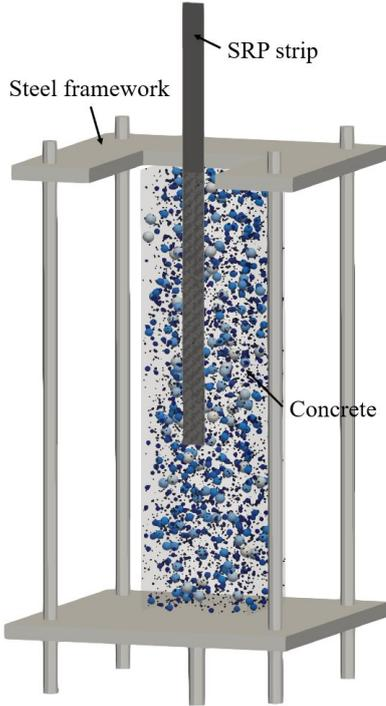
Figure 3: Meso-scale modelling of the single-lap shear test.
