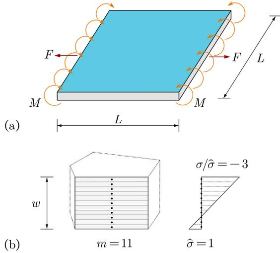
**Figure 2:** Modeling of planar structure under combined membrane and flexural loading: (a) structural layout and loading configuration; and (b) an element cross section and target stress distribution in the thickness direction.
