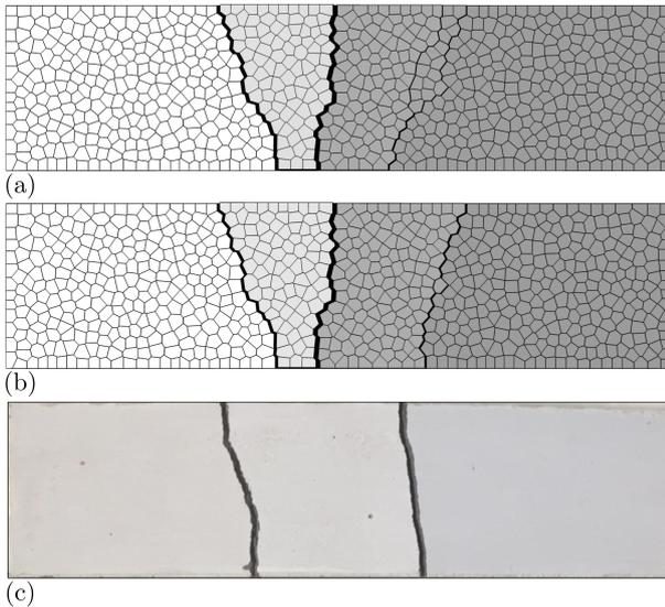
**Figure 7:** Crack patterns obtained from: (a) 3D VCLM analysis; (b) L-VCLM analysis; and (c) physical test specimen with similar wire grid positioning
