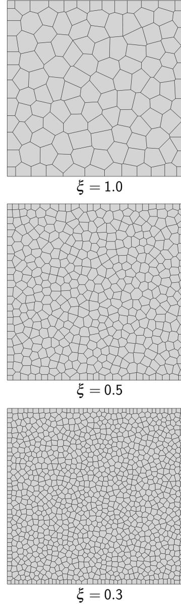
**Figure 3:** Mid-plane domain discretization based on differing average element aspect ratios  $\xi$
