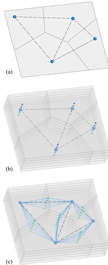
**Figure 1:** Layered Voronoi-cell lattice model: (a) Voronoi partitioning of mid-plane nodes; (b) 3D tessellation based on an extruded set of nodes (c) layered element construction
