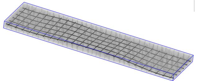
**Figure 5:** Random positioning of a reinforcement layer within the panel specimen model
