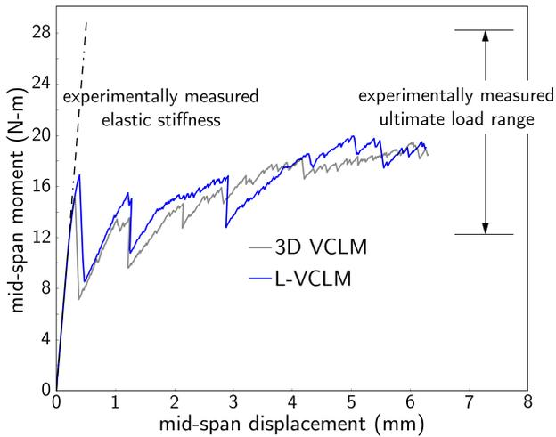
**Figure 6:** Ferrocement panel response to third-point loading
