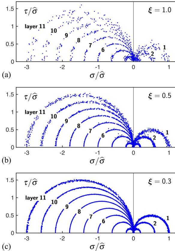
**Figure 4:** Elastic stresses within the planar model under various mesh resolutions: (a)  $\xi = 1.0$ ; (b)  $\xi = 0.5$ ; and (c)  $\xi = 0.3$
