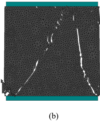
Figure 5: (a) Stress-strain curve for the uniaxial compressive test and (b) deformed specimen (1.5x amplification factor).
