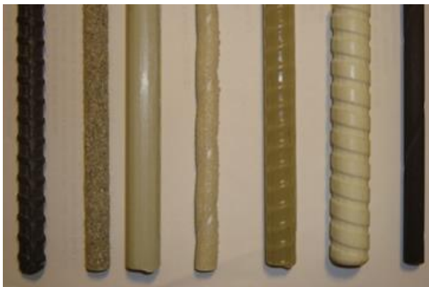
Figure 2. Fibre-reinforced polymer (FRP) bars: Carbon-epoxy (CFRP), glass-epoxy (GFRP), aramid-epoxy (AFRP).
