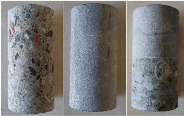
Figure 3: Specimens for uniaxial compressive tests.
