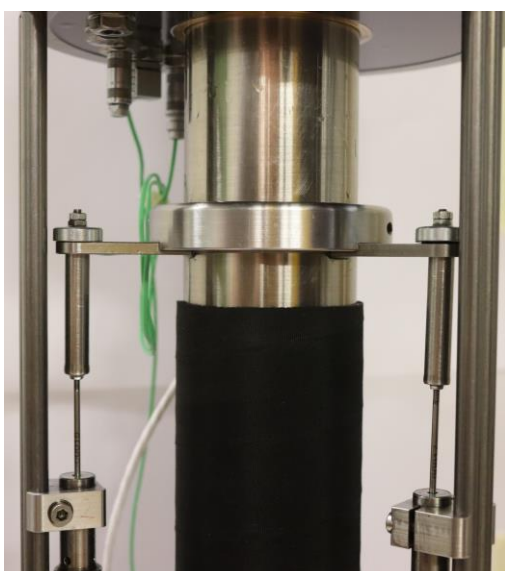
Figure 4: Measurement technology used and internal installation of the triaxial cell
