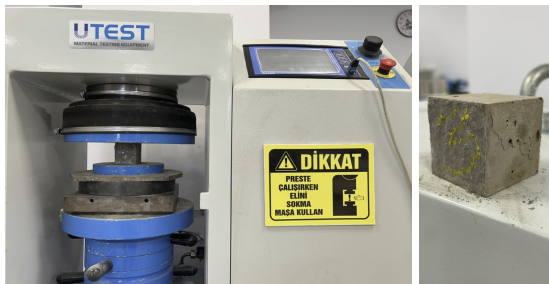
Figure 3: Compressive strength test.
