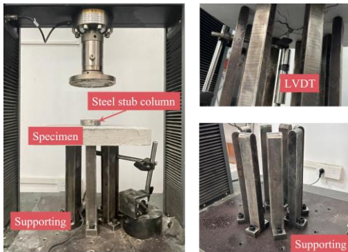
Figure 3: Loading setup and supporting configuration.
