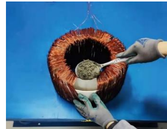
(a) The plastic mould wrapped with copper wire
