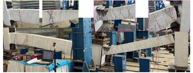
Figure 3: Crack pattern and failure mode of BLPC.
