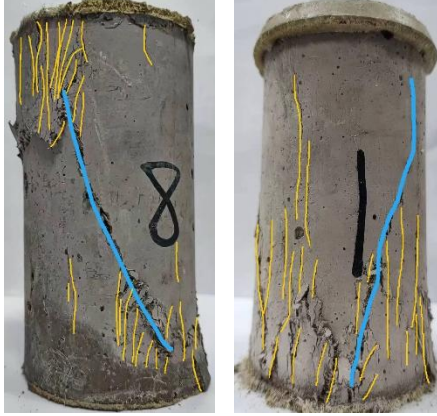
Figure 4: Failure modes of LCC-ECC specimens
