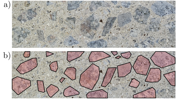
Figure 1: a) A typical concrete mesostructure, b) a possible approximation of aggregates by convex polyhedra.
