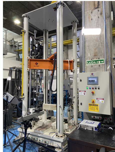
Figure 2: Drop-weight machine at PUC-Rio.
