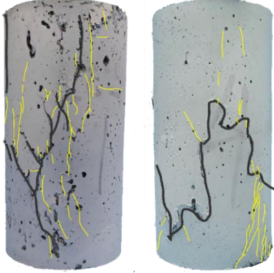
Figure 5: Failure mode of fatigue compression specimen
