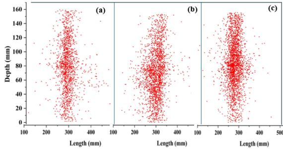
Figure 2: AE events positions of (a) conventional concrete and (b) 0.2% PP fiber concrete (c) 0.4% PP fiber concrete.
