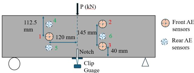
Figure 1: Schematic diagram of three point bending specimen with position of AE sensors.
