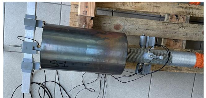
Figure 3: Instrumentation of a model anchor base.
