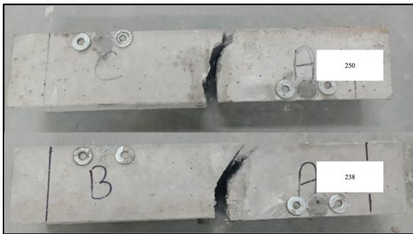
**Figure 5:** Interface cracking and kinking
