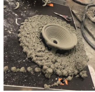
Figure 6: Experimentally-observed failure mode of the studied geometry.
