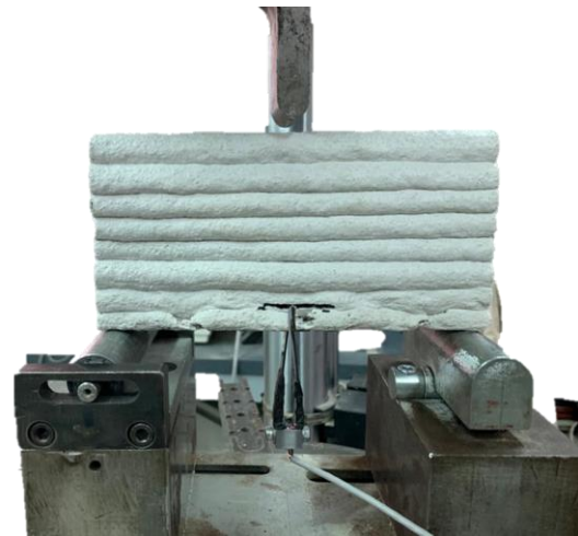
Figure 1: 3-point bending test setup with a clip-gauge at the notch-tip to control CMOD.
