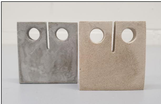
**Figure 2:** Compact-tension (CT) specimen for fracture toughness testing (48 x 50 x 8 mm)
