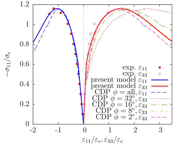
Figure 2: Stress-strain behaviour in equibiaxial compression ( $\sigma_{11} = \sigma_{22}$ ) [42, Fig. 8] with experimental results from [25]. The Abaqus CDP model responses are shown for four values of the dilatation angle. It should be noticed that different dilatation angle gives the best fit to experimental data in comparison to unconfined uniaxial compression (see [42, Fig. 4]) for the CDP model.
