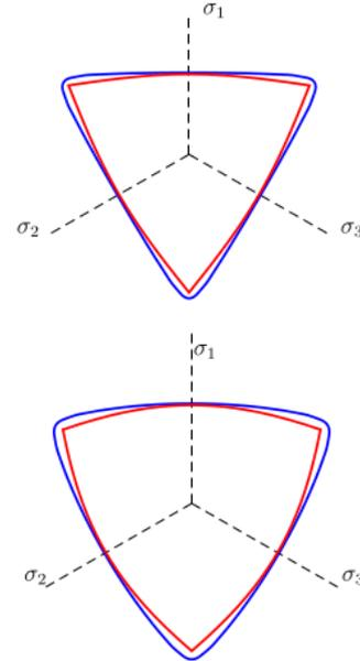
Figure 1: Shape of the failure locus on the deviatoric plane. Above on the  $\pi$ -plane ( $\sigma_m = 0$ ) and at  $\sigma_m = -\sigma_c$  below. Blue curve corresponds to the Ottosen model and red one to the Barcelona model.
