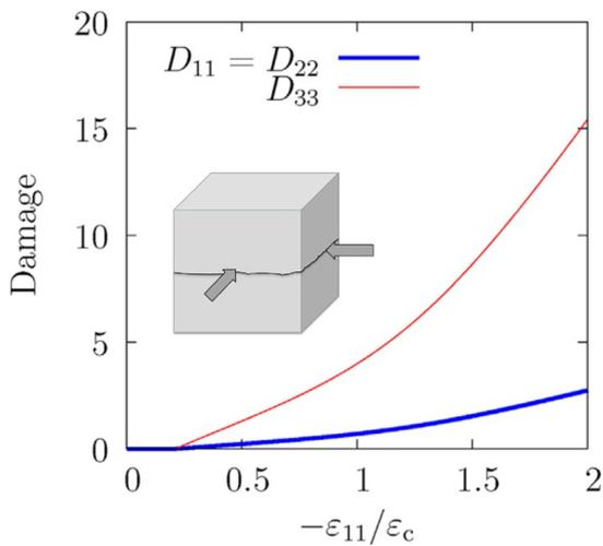
Figure 3: Damage-strain behaviour, damage is the largest in the 33-direction, i.e. the fracture mode corresponds splitting along the compressive plane illustrated [42, Fig.9].
